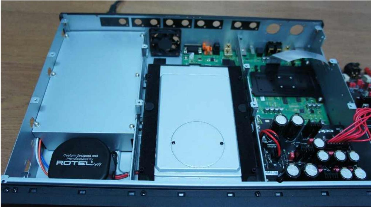
Open upper chassis and take out analog D/A board. You must unscrew many bolts. And take out metal box which covers power module.
