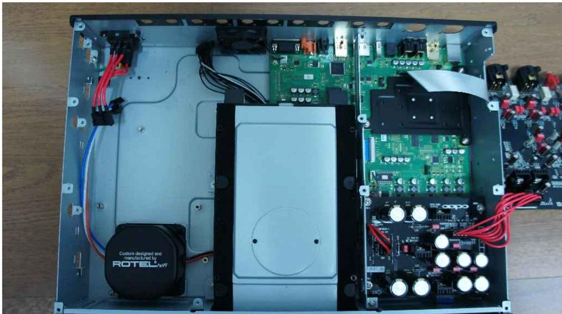
Take out metal bracket which is located between power module and BD rom driver and take out black plastik plate which is under the power PCB sticky ) .
