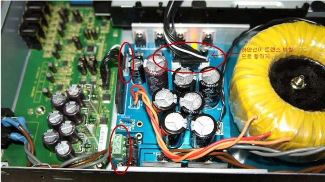
Connect power cord to wall outlet and check whether LED is on. (At this time, don't connect 15 and 6 wires jumper cables).
