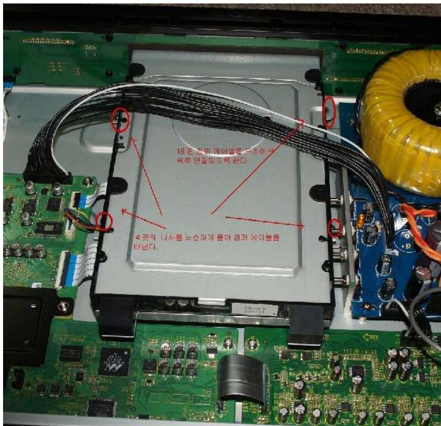
Place 15 wires jumper cable over the Blu ray drive as shown in picture. Loosen the 4 bolts located inside of Blu ray drive to take out 15 wires jumper cable
