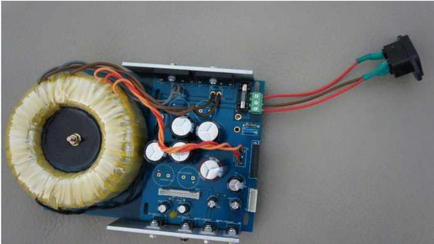
Insert 3 lead wires of power cable to green connector. 2 red ( or orange ) wires should be placed outer socket and 1 brown wire in center socket as shown in picture
